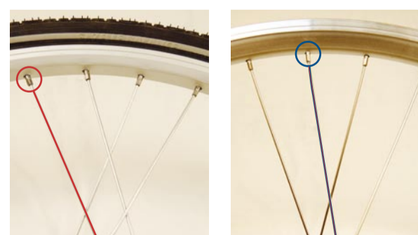
Left: dimpled holes, straight line from nipple to hub. Right: spokes bend just beyond the nipple.
