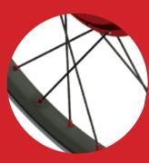
The difficulty with E-Wheel production is the combination of the large hub motor with a standard rim. This way the nipple will not be in line with the spoke. Therefore the rim manufacturers like Rodi, Exal, Remerx and Buchel have invested in the latest Holland Mechanics punching technology for E-rim Solutions. This is done on the High Speed Punching machine whereby they punch
