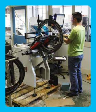
rim with the risk of breaking it and you are certain that the rim has moved the pre-set millimetres ensuring the spoke de-winding has taken place.
