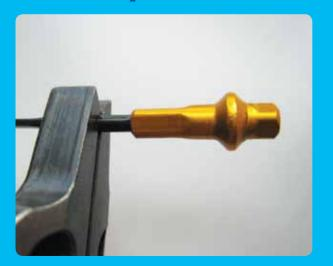
poke Wind-Up; a situation where the spoke gets twisted between nipple and hub is a disaster for high-end wheel building.
