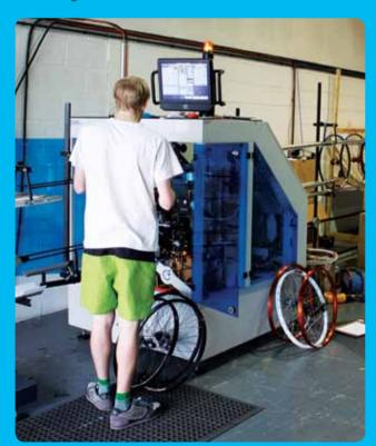
With the recently installed ProLine consisting of an innovative lacing machine with no less than eight nipple containers, in combination with the newest OT Trueing Robot we have lean manufacturing with the maximum flexibility, "said Wilkinson.
